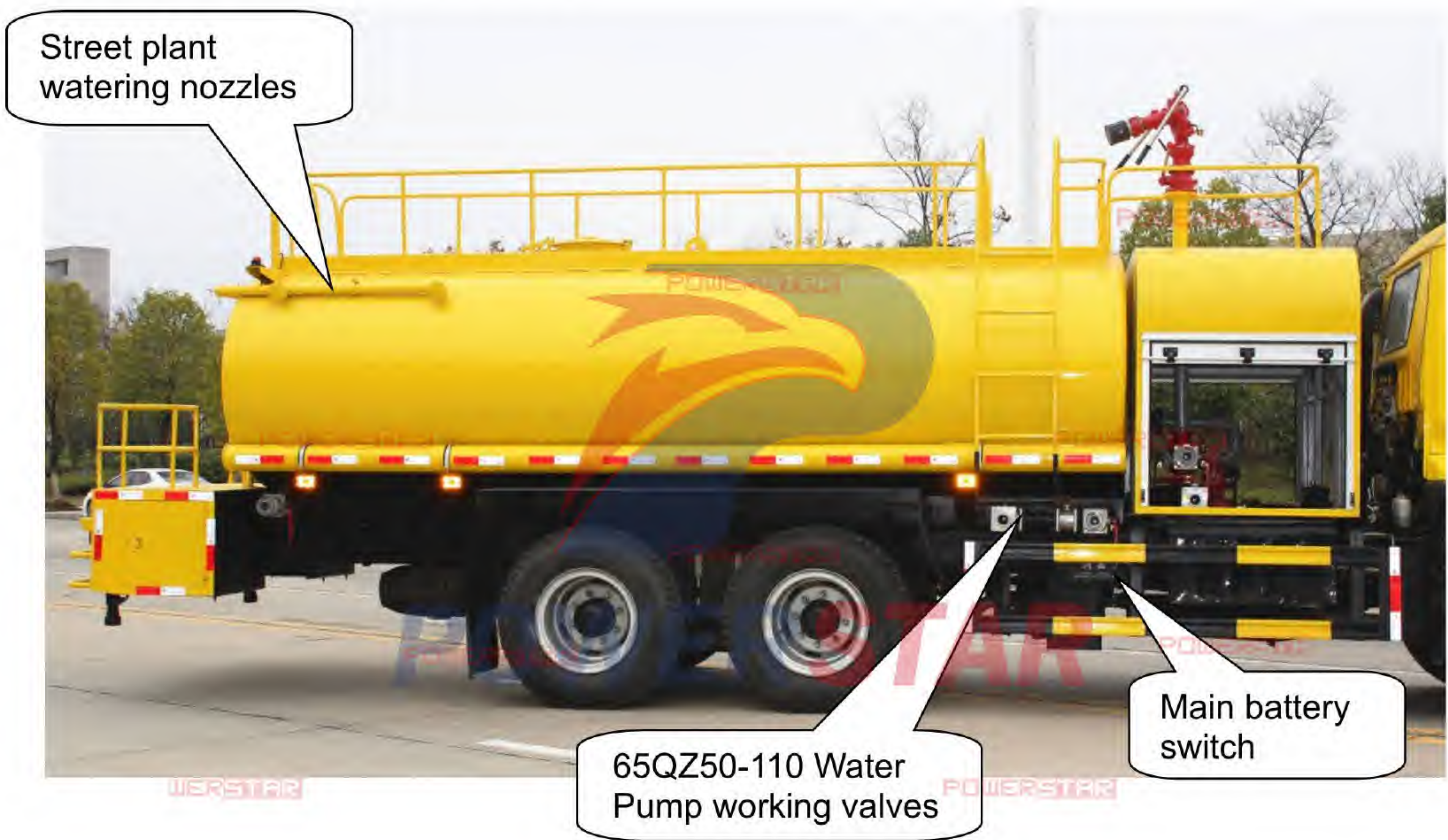
Right side of the Tank (Passenger side): Climbing ladder, fighting house, Pipeline storage box and UQZ (Float Ball Liquid Level Indicator)
